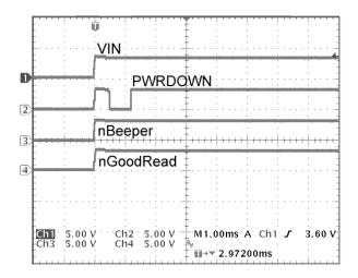
Figure 17. VIN First Applied (USB)
